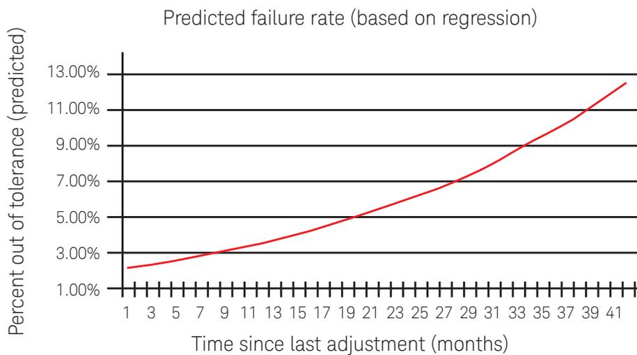
Figure 1. Example of predicted failure rate versus time based on regression analysis of pass/fail data.
